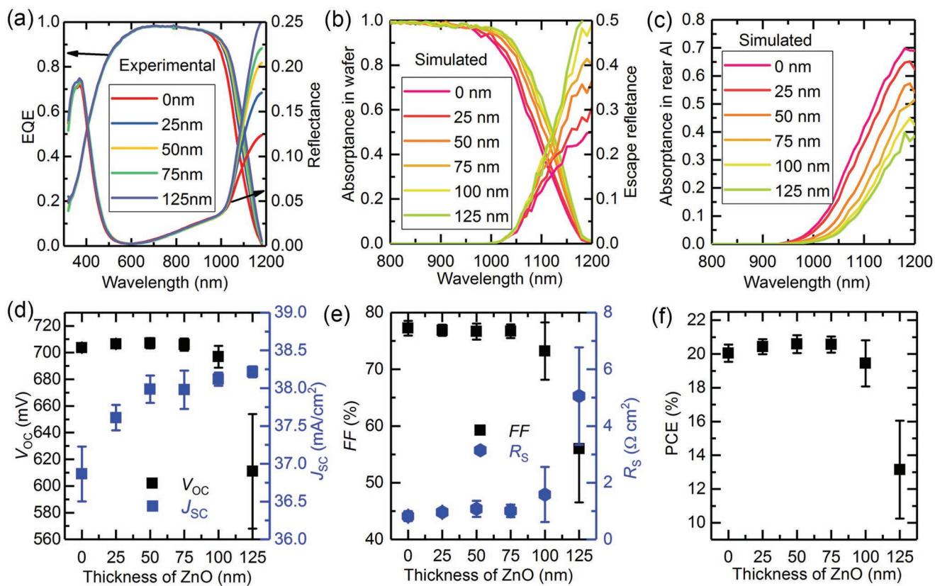
**Figure 3.** a) Experimental EQE and reflectance of the solar cells using different-thickness ZnO layers. b) Simulated absorptance within the Si wafer, internal reflectance and c) absorptance in the rear Al of the solar cells varying with the thickness of ZnO. d)  $V_{OC}$ ,  $J_{SC}$ , e) FF,  $R_S$ , and f) PCE of the solar cells varying with the thickness of ZnO. Note that the label “0 nm ZnO” refers to an electron-selective contact made of a-Si:H(i)/ $\text{LiF}_x/\text{Al}$ .
