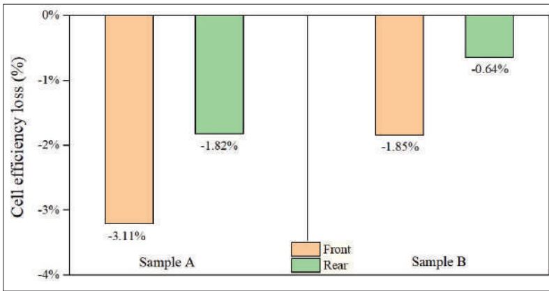
Figure 2. UVID of TOPCon cells from different manufacturers after 30 kWh/m 2 UV irradiation.
